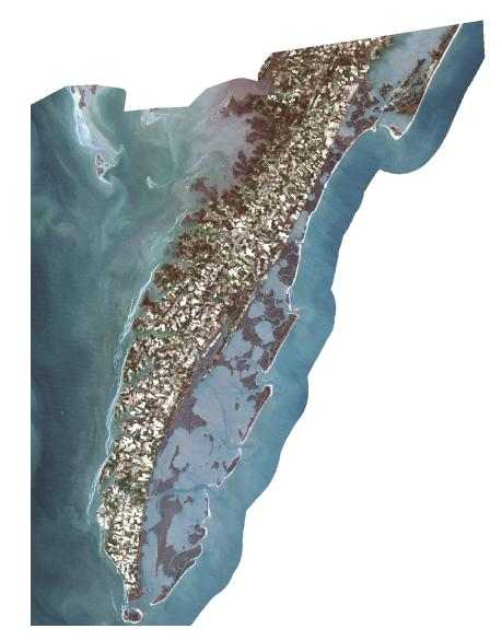
This band combination (321) is referred to as 'True Color' because the red band is displayed as red, the green band is displayed as green, and the blue band is displayed as blue.
