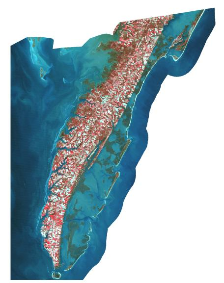
This band combination (432) is similar to color-infrared aerial photography where the near infrared band is displayed as red, the red band is displayed as green, and the green band is displayed as blue.
