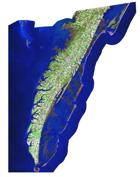
This band combination (542) has mid-infrared band 5 displayed as red, the near infrared band displayed as green, and the green band displayed as blue.
