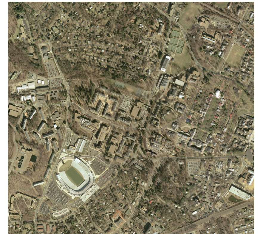
An aerial photograph acquired in March of 2002 as part of the Virginia Base Mapping Project (VBMP). This image is part of a statewide image archive that has a spatial resolution of 1 meter.
