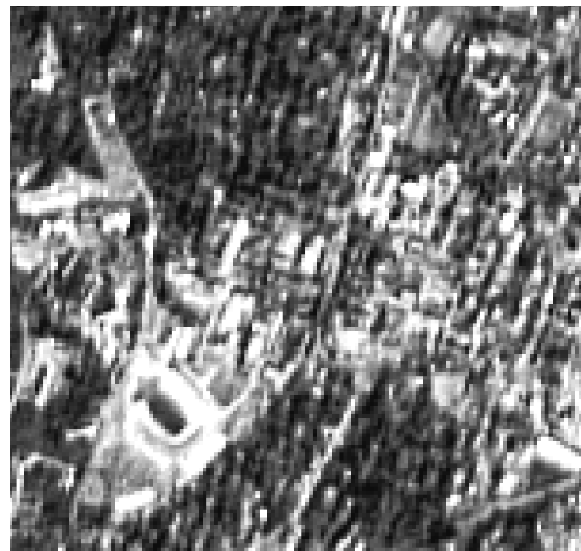
A black and white (also referred to as panchromatic) SPOT satellite image, which has a spatial resolution of 10 meters. The image was acquired on Oct 23, 2000.
